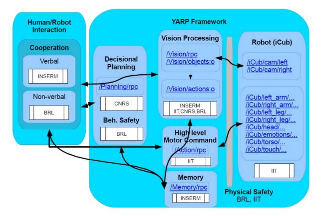
Figure 3 : System architecture synthesis. Note that this figure reflects, as specified in Disclaimer 2, an analysis based on the "integrated platform" demonstration with the iCub. This should generalize across the project, and apply to the largest extent possible to the different platforms including BERT, Jido and HRP2.
