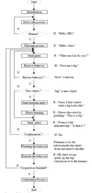
Figure 6. System flowchart of the robot.
