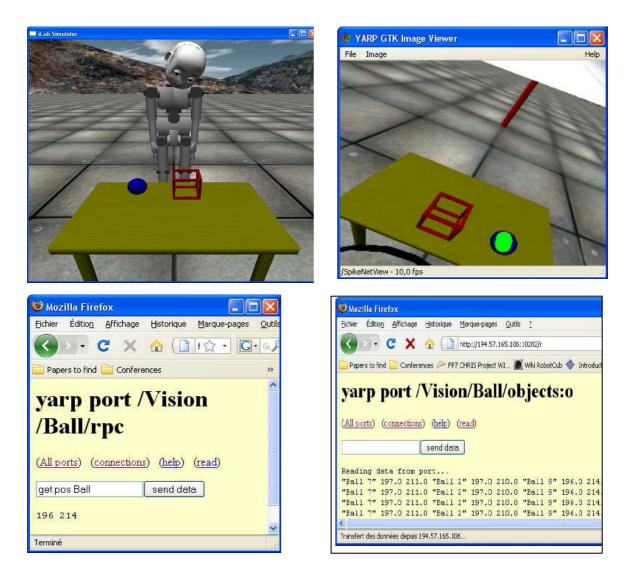
Figure 6. Prototype vision system implemented on iCub simulator. Upper left: robot configuration. Upper right: robot view of table surface, with Spikenet recognition results (green circle) superimposed on recognized object. Lower left: rpc port query and response for recognized ball. Lower right: continuous recognition via :o port.
